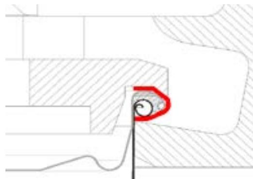
Afterwards the TOPLock tool will press the used sealing unit around the edging of the fuselage.
